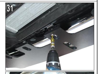
**Fig. 31 until 33**Position the AC Schnitzer front splitter on the vehicle, align and screw tight.
