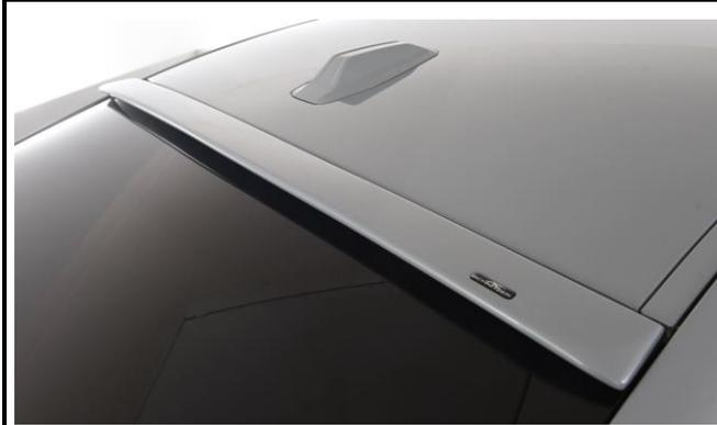
6) Dachheckspoiler / rear roof spoiler
