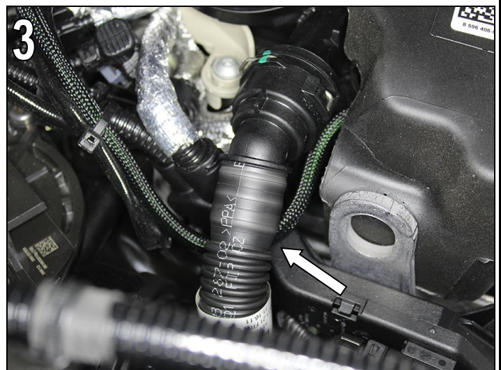
Fig. 3 Route the AC Schnitzer cable harness of the rail pressure sensor below the engine ventilation. To do this, loosen the locking ring of the engine ventilation line and tighten the line.
