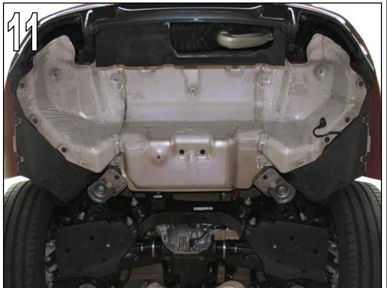
Fig. 11 Release fixing nuts and bolts of the heat shield, and remove heat shield.
