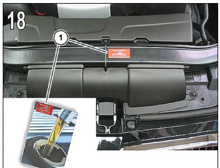
Fig. 18 Affix the stickers (1) in a clearly visible location in the engine bay and in the service book.
